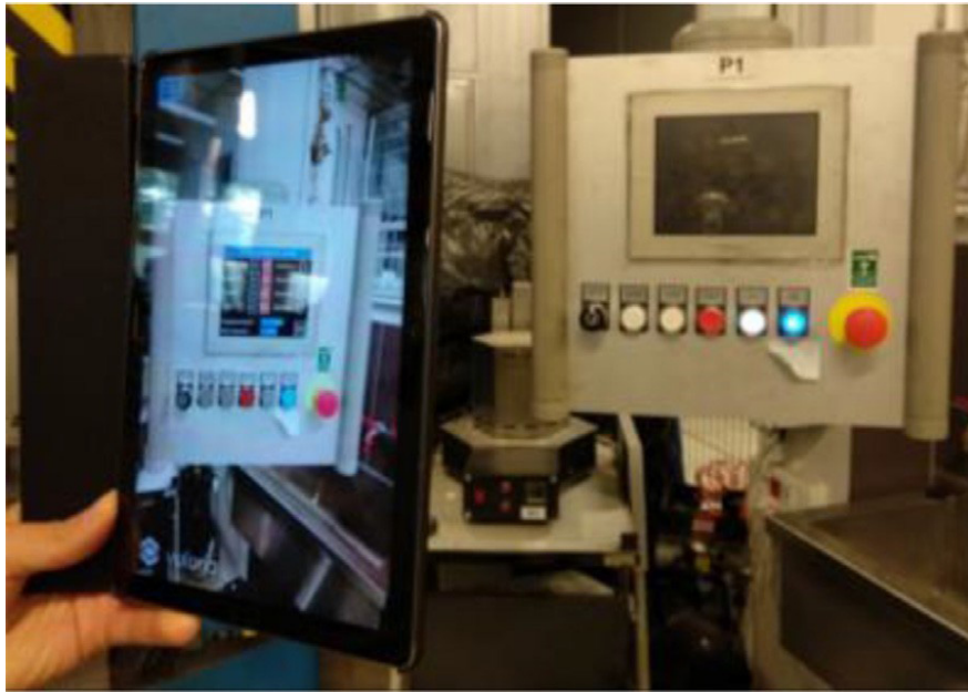
Fig. 43. Augmented reality system of the forging press operation training at AGH University of Science and Technology, Poland.
